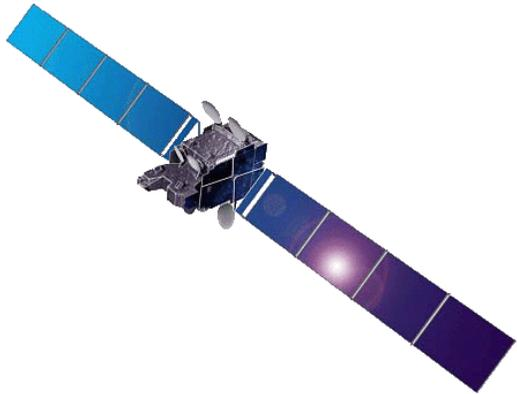
As the demand for satellite capacity has steadily increased, traditional broadcast satellite technology using **Ku-band** (11-14 GHz) frequencies becomes limiting. Because they are built to cover a very large downlink area, traditional broadcast satellites have difficulty supporting the flexible distribution of bandwidth needed for broadband Internet.
