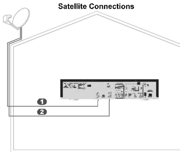
1. Connect two RG-6 coaxial cables between the **SATELLITE IN 1** and **SATELLITE IN 2** ports on the receiver's back panel to two available ports on either your switch or your LNBF in your existing system. See the wiring diagrams in *Chapter 4* for appropriate receiver connections in your system.
