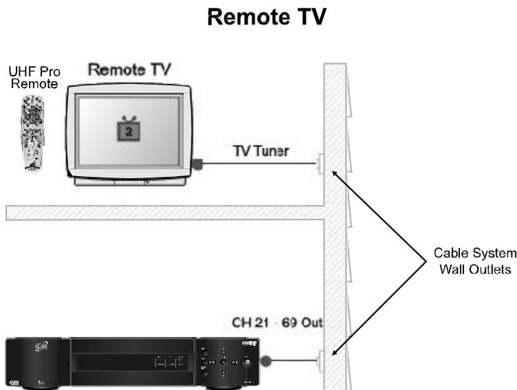
**Note:** When connecting to the home distribution (**CH 21–69 OUT**) coaxial port, you must meet the FCC requirements in the *Appendix*. To meet these requirements, an in-line coaxial attenuator has been included with your receiver and may need to be installed using the following guidance:
