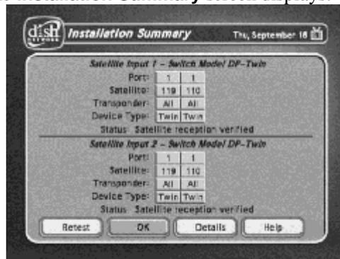
6. Make sure that the information on the **Installation Summary** screen identifies your system correctly and shows all transponders for all satellites in your system. Your screen may look different from the example above depending on the dish antenna system you are using.
