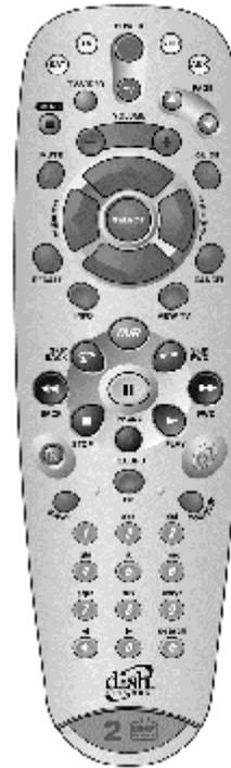
**Remote Control 2** uses UHF Pro signals to control **TV 2** menus for the remote TVs.
